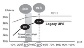
Figure 2: High efficiency at low workload: A high-efficiency UPS uses approximately 5 percent less power than a conventional UPS
